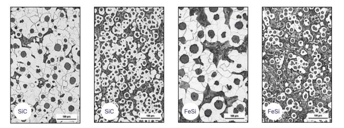
Source: A. VAŠKO. Microstructure and mechanical properties of synthetic nodular cast iron • More nodules in nodular cast iron
