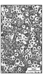
Source: A. VAŠKO. Microstructure and mechanical properties of synthetic nodular cast iron
