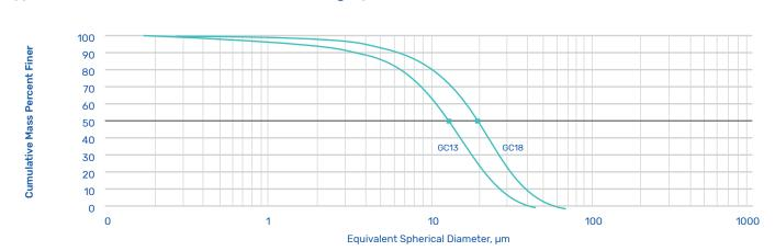
Typical SINTEX sedimentation curves (Sedigraph)
