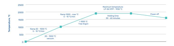
Remarks: Properties given have been achieved on a test specimen that has been pressureless sintered without using a powder bed. A recommended sintering cycle is shown on the above curve. It must be emphasized that the cycle is furnace and load dependent.
